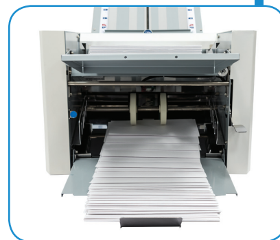
Output conveyor with adjustable stacker wheels for neat, sequential stacking
